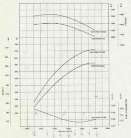
Horsepower, torque, and fuel consumption curves represent performance measured under the ambient conditions of S.A.E. J816b standards.
