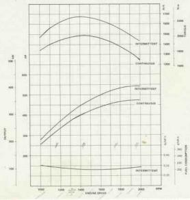
Horsepower, torque, and fuel consumption curves represent performance measured under the ambient conditions of S.A.E. J1349 standards.
