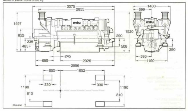
Engine with standard equipment, including coupling and flange-mounted ZF BW 255AP gearbox Mass dry/wet: 3625/3890 kg
