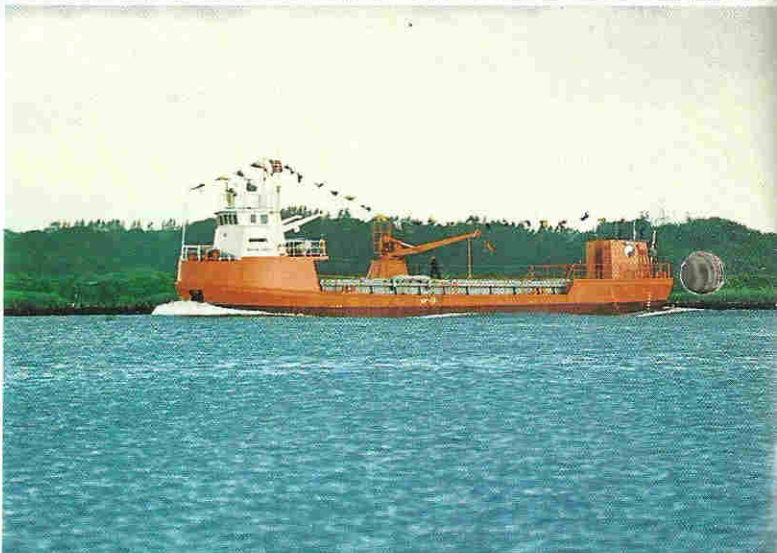
Indian coastguard boat, type SM 45, carrying 2 Scania DSI 11 engines with Hydromat outboard drives. At present there are 20 of these coastguard boats on patrol duties along the Indian coast. All of them are equipped with Scania engines and Hydromat-drives. Max. speed just above 30 knots.
