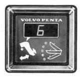
The trim angle is indicated by five green diode lamps plus a digital display. A continuous red light indicates when the drive is in the "beach" sector. The red light flashes when the drive is in the
